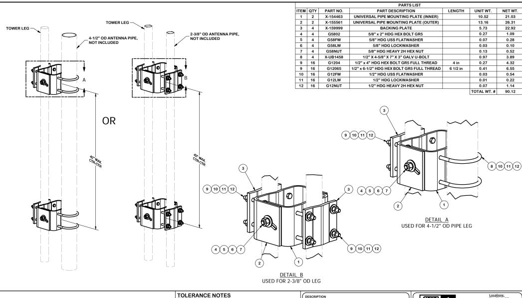
TOLERANCES ON DIMENSIONS, UNLESS OTHERWISE NOTED ARE: SAWED, SHEARED AND GAS CUT EDGES (\$ 0.030") - NO CONING OF HOLES LASER CUT EDGES AND HOLES (\$ 0.030") - NO CONING OF HOLES
